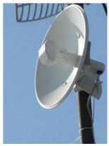
Fig. 10. The client station of a communication network NSSM for long distances
