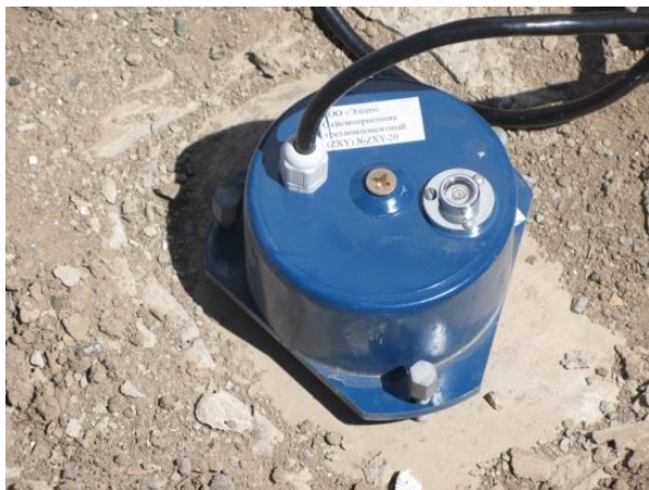
Fig. 10. Installation of the geophone on the concrete foundation
